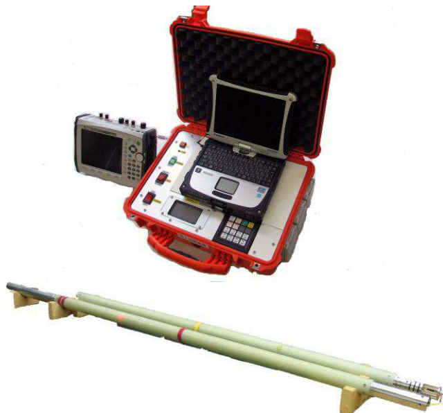
Fig. 1. Carrying case including ground surface electronics, portable VNA, and laptop computer (top). Transmitter and directional probes with a diameter of 57 mm (bottom).
