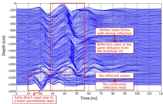
Fig.3 Similar reflected waves down to a depth of about 22 m and turbulent waves around the bottom.
