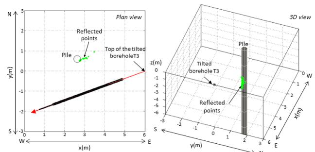
Fig. 6. The 3-D reflected points with the pile's actual position estimated from RT measurements in the tilted borehole T3.
