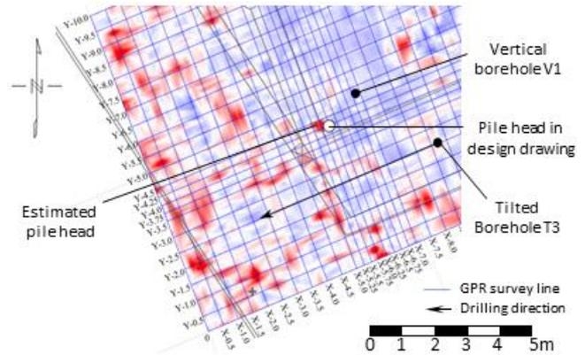
Fig. 1. Strength distribution of radar waves reflected from depths of 0.8 to 0.9m.
