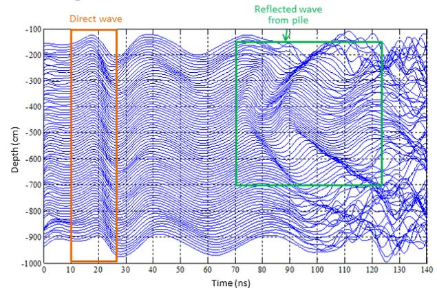
Fig. 5. Strong reflection obtained at tilted measurement borehole T3 (central frequency of bandpass filter: 100MHz; bandwidth: 100MHz).
