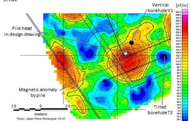
Fig. 2. Analytic signal of vertical gradient of the magnetic field.
