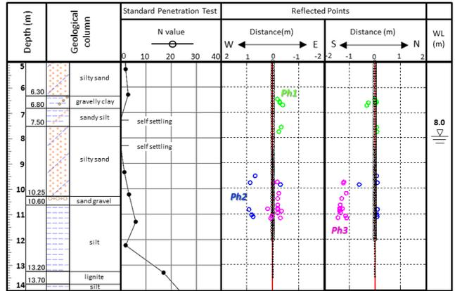
Fig. 9. Reflected points on two sections and geological column with N-values of the measurement borehole N1.
