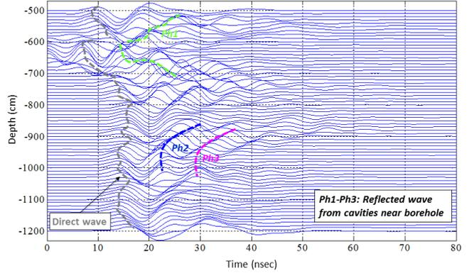
Fig. 8. Complicated radargram with several reflection waves.
