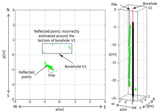
Fig. 4. The 3-D reflected points with the pile's actual position estimated from RT measurements of the vertical borehole V1.
