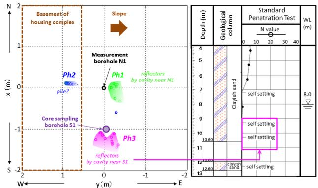
Fig. 10. Planar view of reflected points with geological column and N-values of the core sampling borehole S1.
